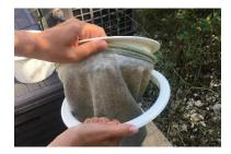
Then take another (clean) filter bag and put it on the rings as the other one came off. So first the large ring over the bag and the small ring in the bag. Then push the large ring back over the small ring.
